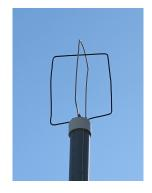
EggNOGS is an Egg Bearter antenna kit, for working satellites.
